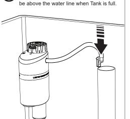
Connect the Refill Tube Clip to the Flush
