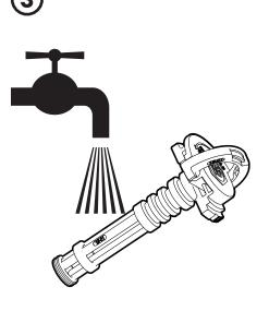
Clean Filter by rinsing under running water.
