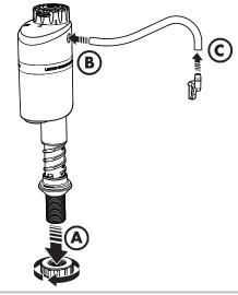
Position the Fill Valve within the Toilet Tank. Properly align the Fill Valve so there are no kinks in the Refill Tube, and so there is proper clearance to the Flush Handle Rod (A). From below, install the Quick Connect Mounting Nut by pressing upwards until the Nut makes contact with the Tank (B). Then hand tighten secure
