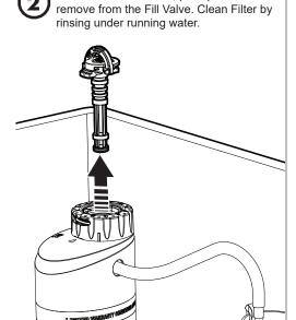
Once Filter is released, pull upward to
