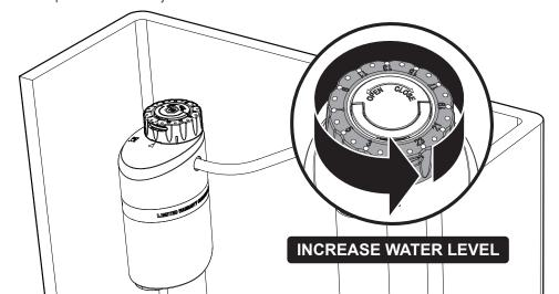
This Fill Valve is factory set to the lowest water level. To **DECREASE THE WATER LEVEL IN** TANK, hold the Body of the Fill Valve stationary and rotate the Top Dial clockwise until the desired water level is achieved. There are 24 indicators dots on the Top Dial that each represent a
